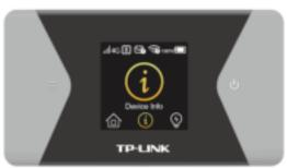
2) Press the Power button to select it and enter the Device Info Screen. You can find the SSID here.
