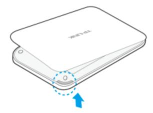
2) Slide and lift up the SIM card slot cover.
