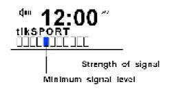
The indicator on the signal bar shows the minimum acceptable signal level.
