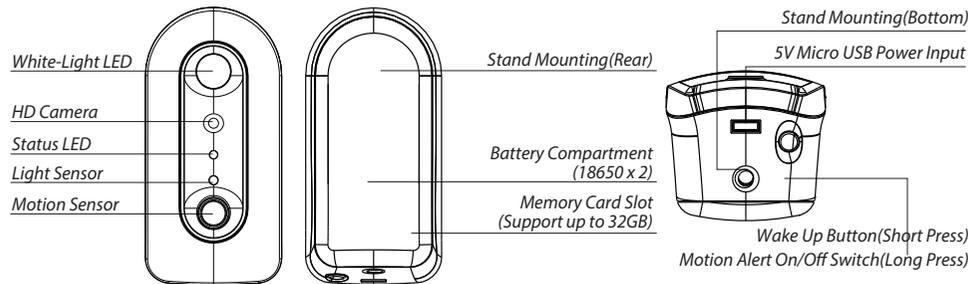
To Activate Motion Alert: Long press for 5 sec until Red LED blink once
