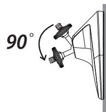
**3 Adjust proper view angle, then secure the joint with T-bolt.**
