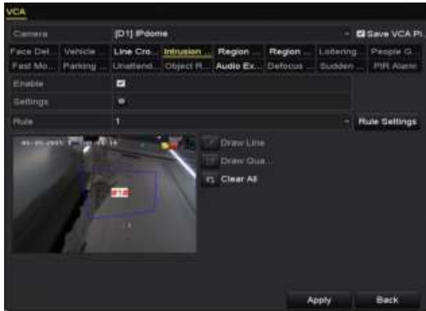
Figure 10-9 Draw Area for Intrusion Detection
