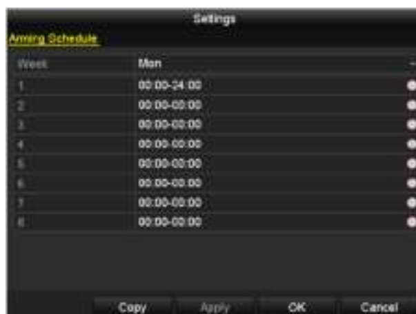
Figure 8-20 Set Arming Schedule of Alarm Output
