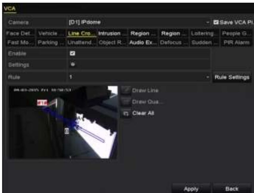
Figure 10-7 Draw Line for Line Crossing Detection
