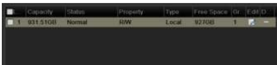
Figure 14-4 HDD Status Changes to Normal
