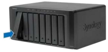
3 Pull the hard drive tray handle in the direction as indicated below to remove the hard drive tray.
