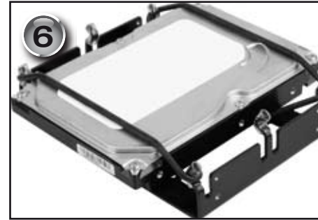
6. Slide the outer string of the second rubber band over the HDD and center the drive between the rubber bands (fig. 6).
