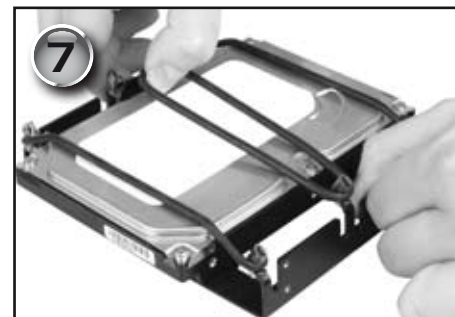
9. Fasten the last rubber band to the frame's central hook (fig. 7).
