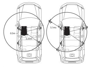
The sound is not balanced because the distance between the listening position and the various speakers is different.
