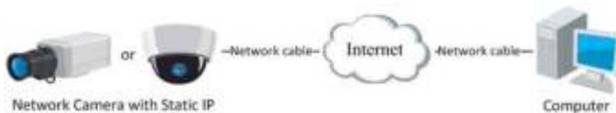
Figure 2-5 Accessing the Camera with Static IP Directly
