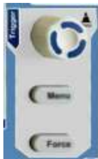
Figure 3-12 Trigger Control Zone
