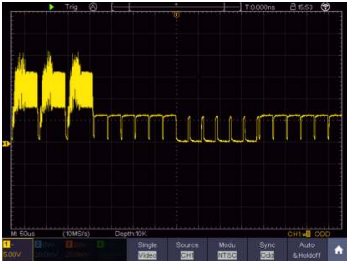
Figure 9-7 Waveform Captured from Video Field Trigger
