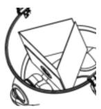
• Attach the top of the vacuum cleaner to the collection container and secure it with the indicated hook.
