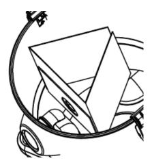
• Attach the top of the vacuum cleaner to the collection container and secure it with the indicated hook.
