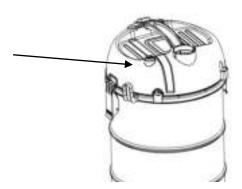
• Release the hook and lift the cover of the vacuum cleaner.
