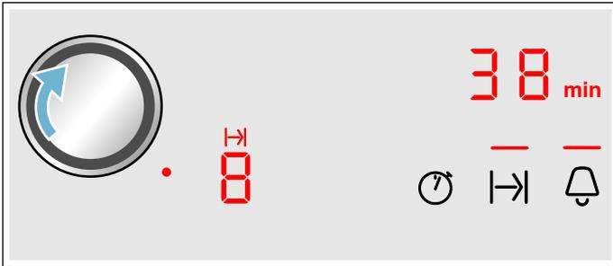
The cooking time counts down. If you have set a cooking time for several cooking positions, the shortest cooking time will be displayed. — above the I→I symbol lights up. The I→I display for the cooking position lights up.
