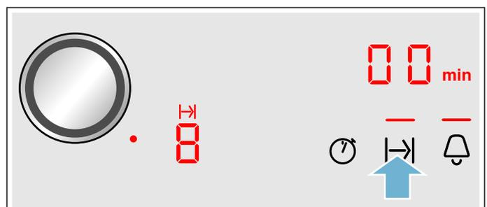
3. Within the next 10 seconds, set the desired cooking time with the twist knob.
