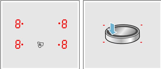
The twist knob is magnetic and is placed on the twistpad. Tapping the twist knob where there is a marking activates the relevant hotplate. Turning the twist knob selects the heat setting.
