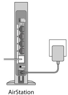
5 If using a wired LAN, connect the AirStation LAN port and computer using a LAN cable. If using a wireless LAN, connect the computer to the wireless LAN as described in Chapter 3.
