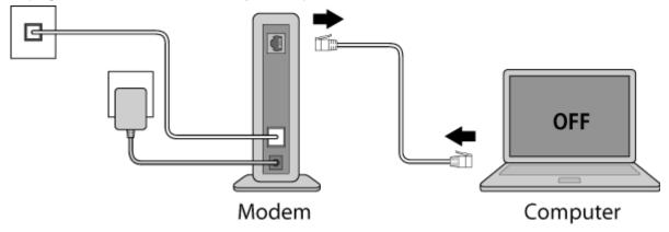
3 Confirm that the mode switch is in the "Auto" position. Plug one end of the LAN cable into your modem and the other end to the AirStation's Internet (WAN) port. Turn on the modem.
