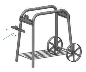
Assemble the lid with 1pcs M6\*20 step screws
