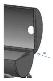
2.10 Assemble the smokestack with 2pcs M6\*12 screws and 2pcs M6 nuts
