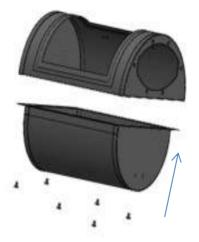
16 Assemble the side box with 8pcs M6\*12 screws and 2pcs M6 nuts
