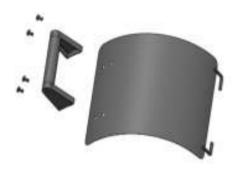
2.21 Assemble the Front shelf with 6 2.22 pcs M6\*12 screws and 2pcs M6 nuts
