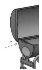
Assemble the side box bracket with 2pcs M6\*12 screws
