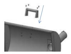
Assemble the side box with 6pcs M6\*12 screws
