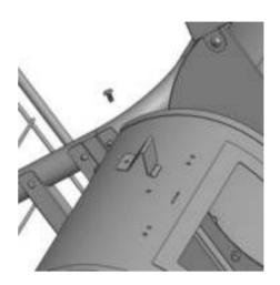
2.20 Assemble the side box lid with 4pcs M6\*12 screw 4pcs and M6 nuts(usually this part was assembled)
