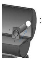
2.11 Assemble the smoke stack lid with spring (usually this part was assembled)
