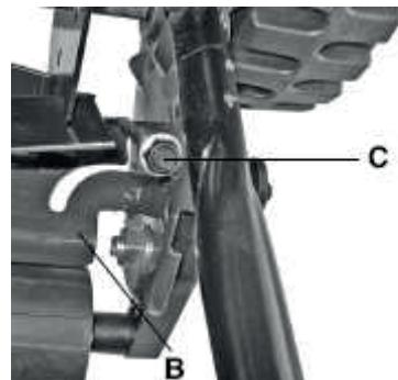
**Note:** The counter blade (B) is only be adjusted before using the machine for the first time or if the blades on the mower spindle are worn.
