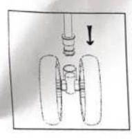
2. To install the front wheel, insert wheel onto the leg until a "click" is heard.
