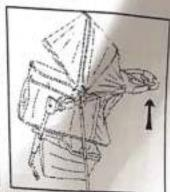
1.Release the red locking latch, unfold the stroller upwards and make sure both locks nap into place.
