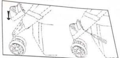
5. To attach footboard position to bottom as shown and tighten screws.
