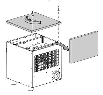
2. Clean the filter using a slightly damp, soft, lint-free cloth. If the filter is heavily contaminated, clean it with warm water mixed with a neutral cleaning agent.
