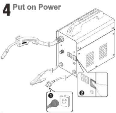
2 Power switch, switch On/ Off
