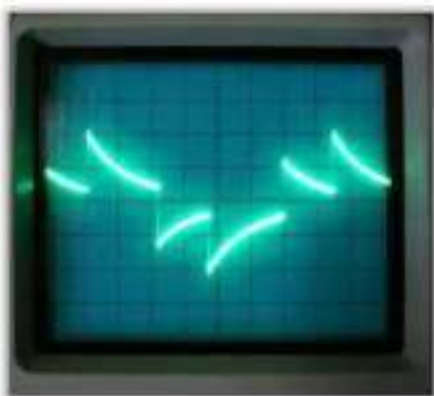
Modified Sine Wave and Pure Sine Waves on Oscilloscope
