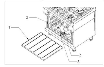
To replace the heating elements in the oven, extract the steel rod grill, the base (1), the upper diffuser and the grill holders. Then loosen the screws (2) holding the element to be substituted (3); detach the heating element from its support on the opposite side; remove it, together with the wiring, and disconnect it.
