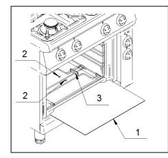
In order to replace the oven heating elements, extract the oven grill, the floor (1), and the grill holders. Then, unscrew the fixing screws (2) of the heating element to be substituted (3); remove the heating element from the support from the other side; remove it, including the wiring, and disconnect it. Then, connect the electric cables following the instructions of the wiring diagram.
