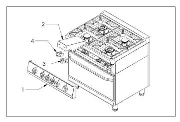
To replace the selector (4) and the thermostat (3) in the electric oven, loosen the fixing screws on the control panel (1) and the protective hood (2) and remove them. Then disconnect the electrical wiring on the component and replace it. Then reconnect the electrical wiring following the instructions on the wiring diagram.
