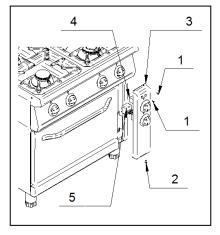
Electric components of the electric oven
