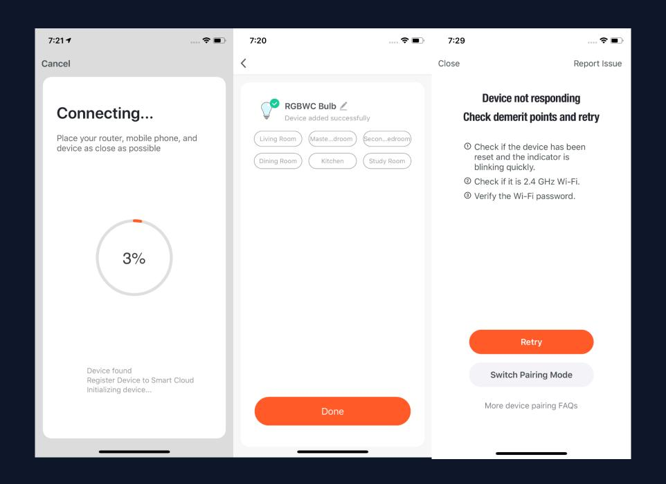
5. If want to you use EZ mode to connect your devices, the process is presented in the first two pictures on the left. You can customize the names of the devices (64 characters maximum) and assign rooms for the devices. 6. If it fails to connect the device, the app will show the third page on the left. You can follow the instructions to solve the problems.
