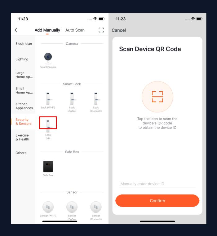
**Choose the NB** products you want to connect and click the scan icon on the upper right corner to scan the device's QR code. Or you can directly enter the IMEI number on the device's label and choose "Confirm" to connect the device with the app. (The app will need phone camera access when scanning.)
