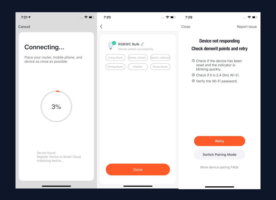
8. Connect to the device's hotspot and return to the network configuration page in the app to continue the process. The page will appear as shown in the pictures to the left. After the devices are successfully connected, you can customize their names (64 characters maximum) and assign rooms to them.
