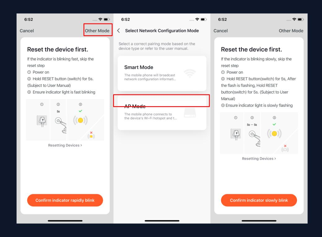
1. There are two network configuration modes for devices (except IPC devices and NB devices): EZ mode and AP mode.
