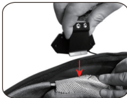
Fig.3 Adjust the position of Bluetooth core from left to right Then lock the upsetting wire and fix it.
