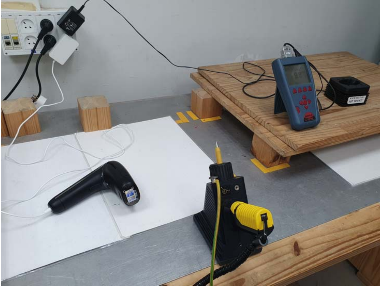
Picture # 23. ESD Immunity test setup – tested points. Contact ESD to Touch panel
