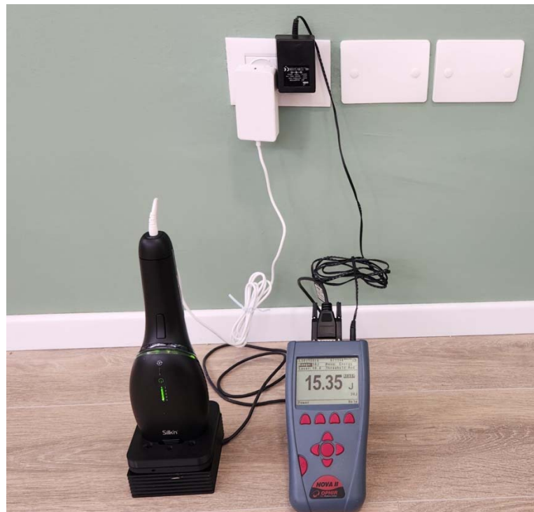
Picture # 7. Light pulse energy measurement test setup
