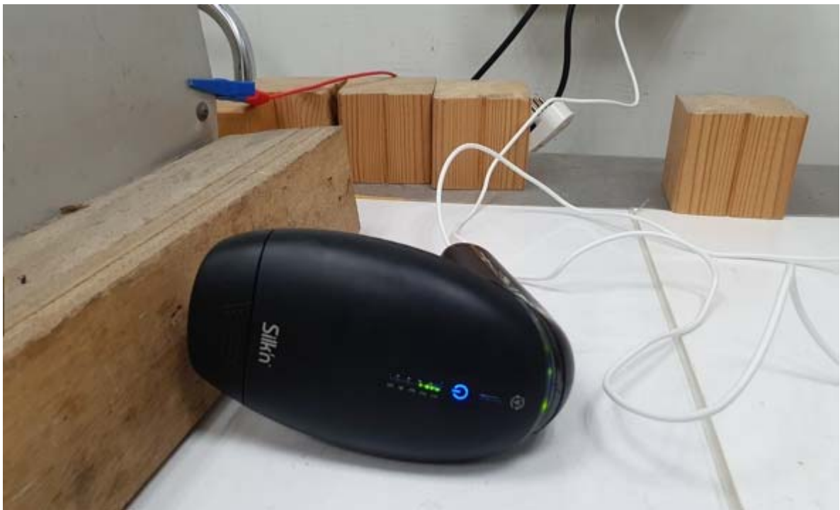
Picture # 20. ESD Immunity test setup – tested points. Contact ESD to VCP/HCP planes
