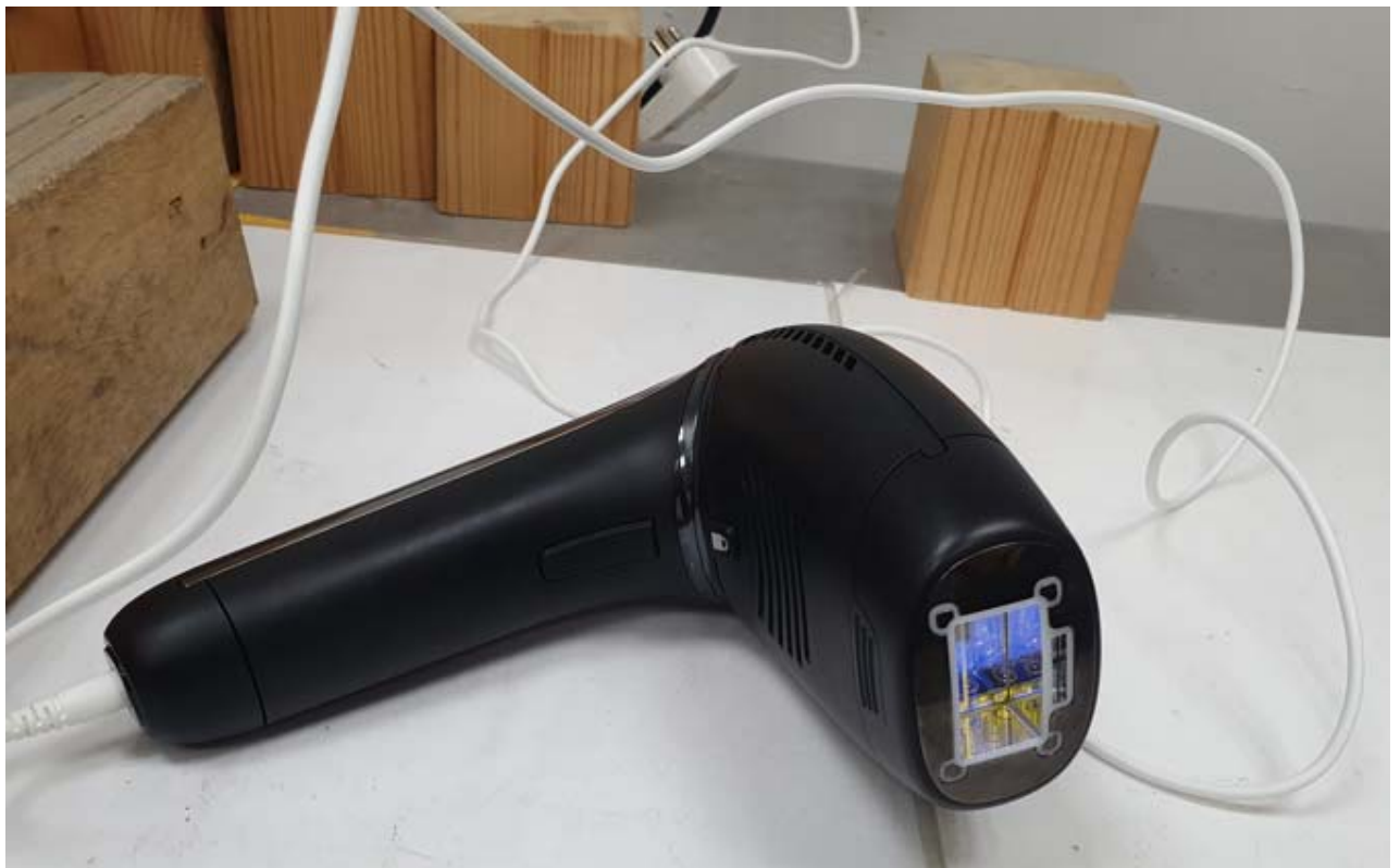
Picture # 21. ESD Immunity test setup – tested points. Contact ESD to Touch panel
