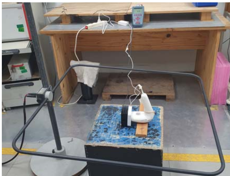
Picture # 16. Magnetic field immunity test setup per IEC 61000-4-8
