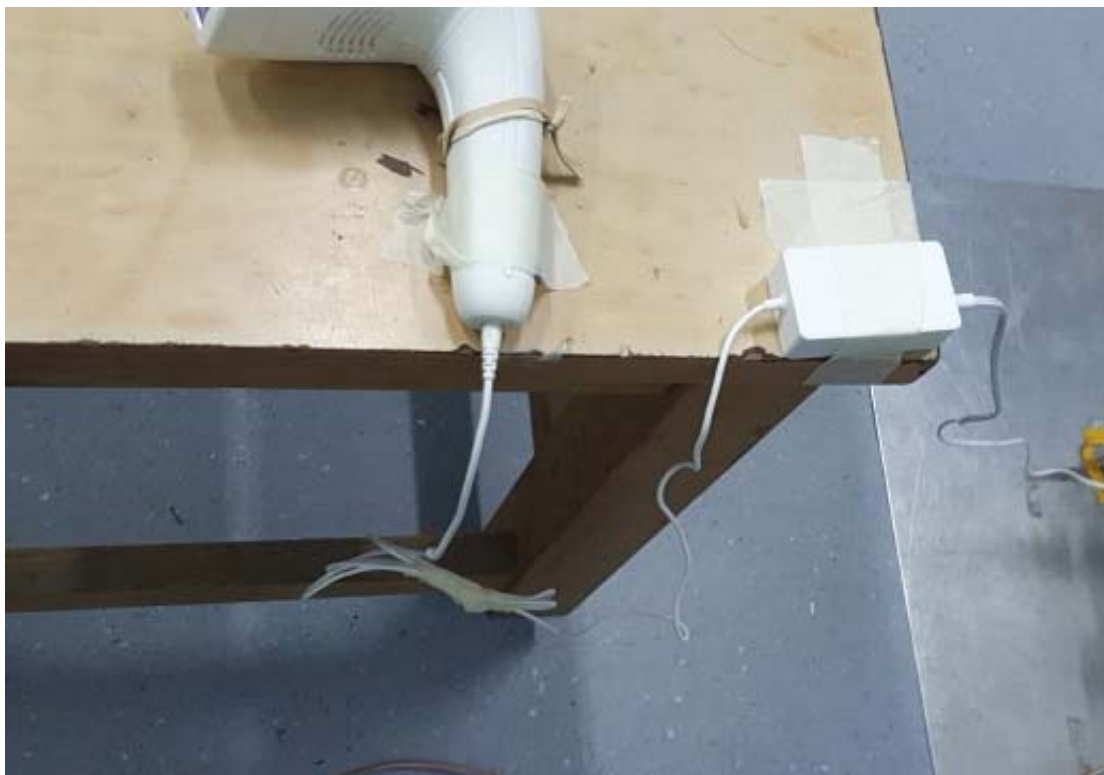
Picture # 9. Conducted emission test setup
