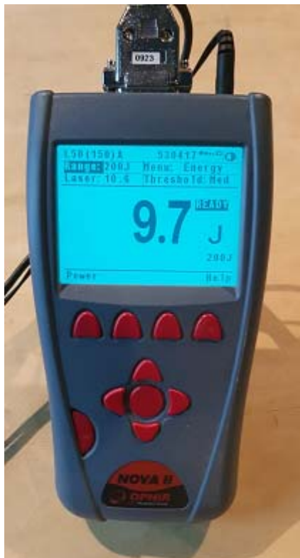
Picture # 12. Radiated Immunity test setup. Light pulse energy reading on OPHIR – NOVA II
