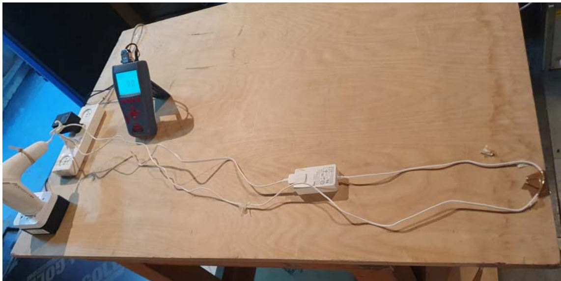
Picture # 11. Radiated Immunity test setup per IEC 61000-4-3
