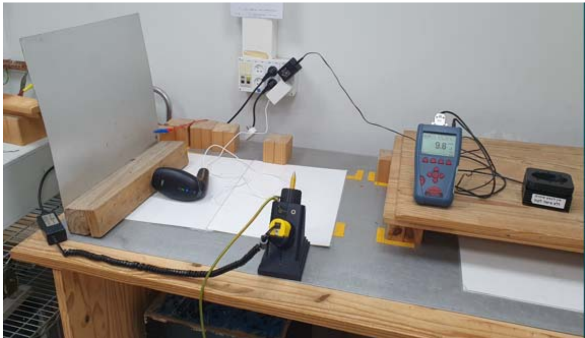
Picture # 19. ESD Immunity test setup per IEC 61000-4-2. Contact ESD to VCP/HCP planes
