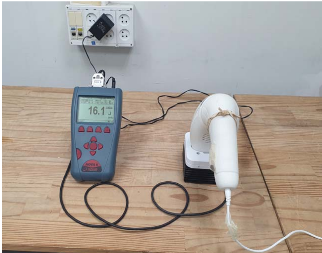
Picture # 15. Voltage dips/interruption test setup on AC mains per IEC 61000-4-11
