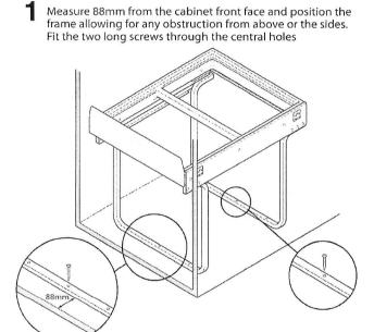
Before permanent attachment to the cabinet base, fit containers and lid and test for ease of opening and container removal. Ensure the unit is clear of door hinges and other obstructions during operation.
