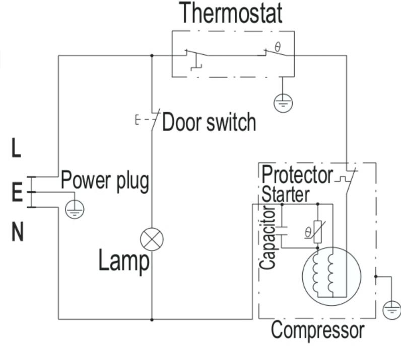
Capacitance is chosen according to the compressor
