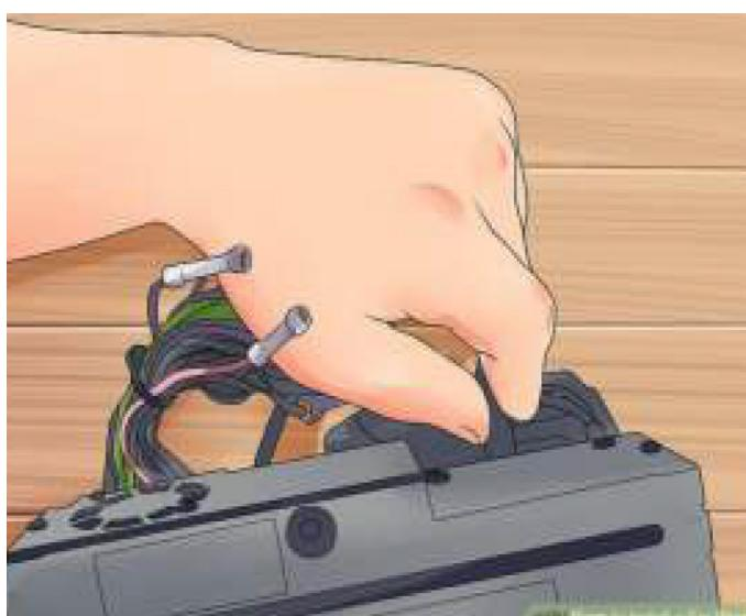
Connect the power source. if you have a wiring harness, this connection is made when you connect the new stereo harness to the wiring harnesses in the car.
