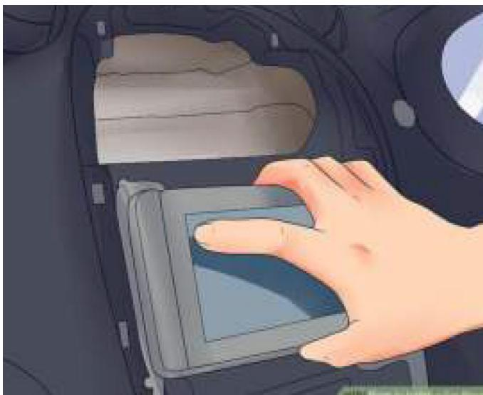
Push the stereo into place. If the stereo is fully seated you should hear a click.
