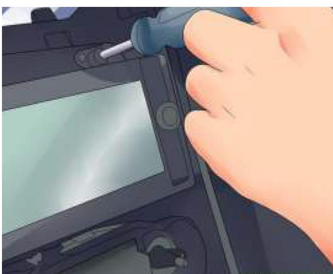
Attach all screws that are needed to hold the stereo system in place, reconnect all wired components again and reinstall any knobs or drawers that were removed back in place.
