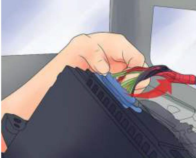
Disconnect the stereo connectors. there is a series of wires connected to the back of the stereo, and you need to disconnect them all. First, disconnect the antenna wire, which is usually a thicker wire connected separately from the rest. once this is disconnected, you can move the stereo more freely move.
