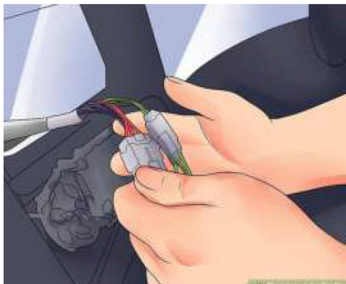
If you are using a wiring harness, this connection is made when you connect the parts of the bundle connect.
