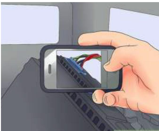
Take a picture of how the stereo is connected. this is an important step because the photo will later serve as a reference when you connect the new stereo.
