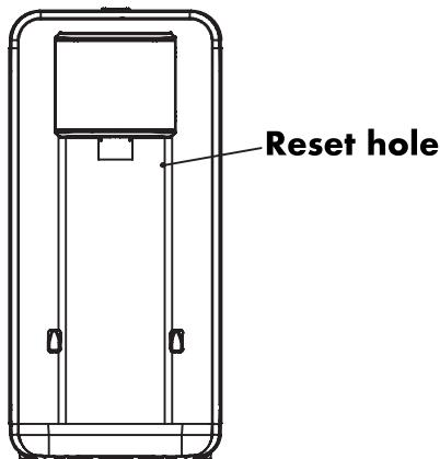
The appliance has a manual thermostat to recover the heating function for abnormal operation, if the unit is no power, stop working, not boiling the water, you can reset the thermostat by using the reset key to press the reset hole.
