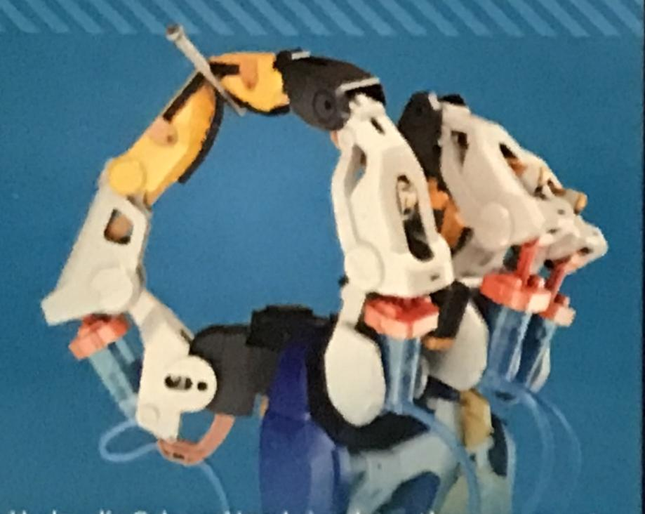
The Hydraulic Cyborg Hand simulates the movements of a human hand using hydraulic power for mechanical transmission without electricity. It allows every finger joint to adjust at different angles for a precisely closed fist or open palm.
