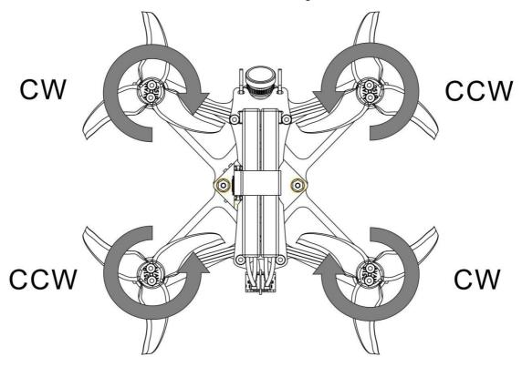
**Caution:** Failure to mount the propellers in the correct orientation will cause Tinyhawk II Freestyle to not fly correctly and with no control. Please double check for the correct orientation.
