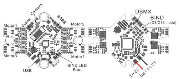
Tinyhawk II Freestyle's main electronic board is shown above. This board contains a F4 flight controller with all 4 esc's and an 8CH receiver.
