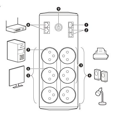
Connect a master device, such as a desktop computer or audio/visual receiver to the Master outlet. Connect peripheral devices such as a printer, speakers, or a scanner to the Controlled outlets.
