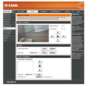
Preset List: To add a preset to the sequence, select it from the drop-down box at the bottom of this window, set the Dwell time to determine how long the camera view will stay at that preset, then click the Add button. The preset name will appear in the list, followed by the dwell time to view that preset for.
