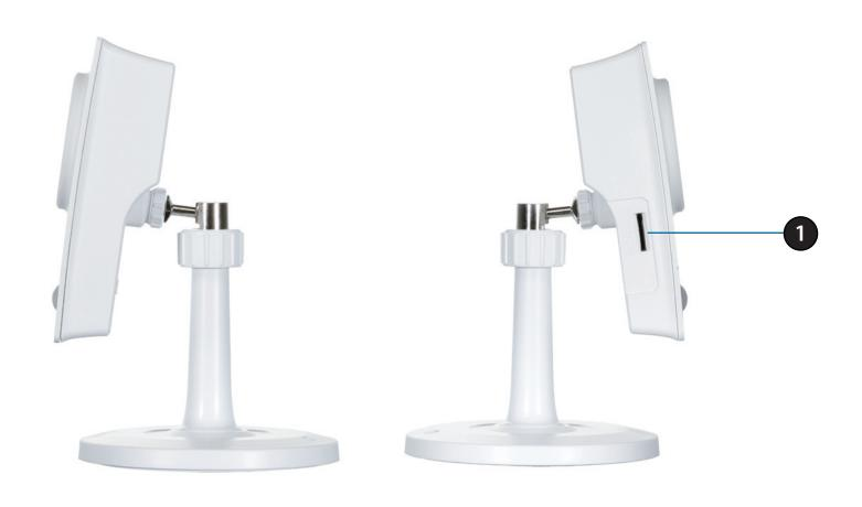
1 Micro SD Card Slot Insert a MicroSD card for Local storage for storing recorded image and video
