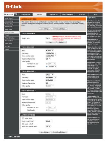
Maximum frame rate: A higher frame rate provides smoother motion for videos, and requires more bandwidth. Lower frame rates will result in stuttering motion, and requires less bandwidth.
