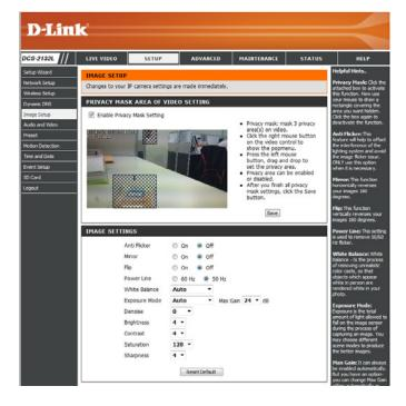
Exposure Mode: Changes the exposure mode. Use the drop-down box to set the camera for Indoor, Outdoor, or Night environments, or to Moving to capture moving objects. The Low Noise option will focus on creating a high-quality picture without noise. You can also create 3 different custom exposure modes. The Max Gain setting will allow you to control the maximum amount of gain to apply to brighten the picture.
