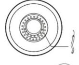
Use the Iron wire to help the water passing through the small holes
