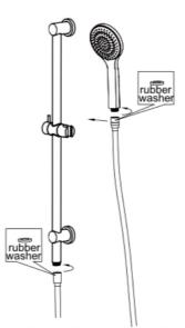
5. Connect shower rail and hand shower with hose. TEST & CHECK FOR LEAKS.
