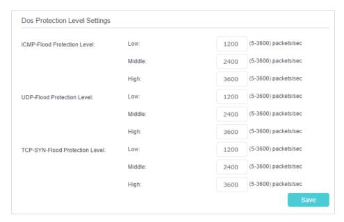
2. The protection will be triggered immediately when the number of packets exceeds the preset threshold value, and the vicious host will be displayed in the Blocked DoS Host List.
