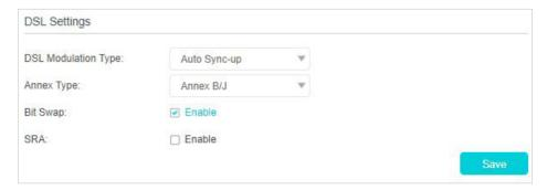
3. Select a DSL Modulation Type/Annex Type from the drop-down list. Do not change the default settings unless necessary.
