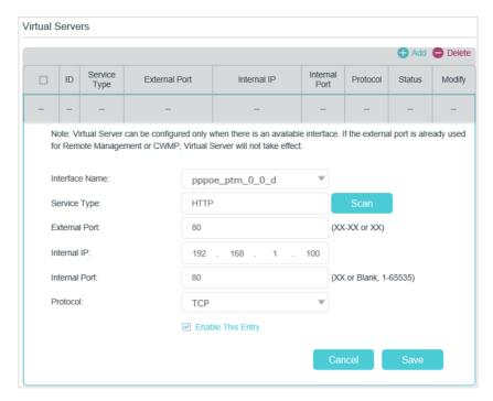
Click Scan, and choose HTTP. The external port, internal port and protocol will be automatically filled with contents. Enter the PC's IP address 192.168.1.100 in the Internal IP field.
