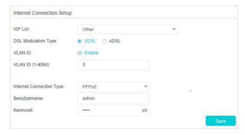
3. Click Save to make the settings effective, and you can refer to <u>Test Internet</u> <u>Connectivity</u> to test the internet connection.
