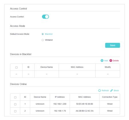
3. Select the access mode to either block (recommended) or allow the device(s) in the list.
