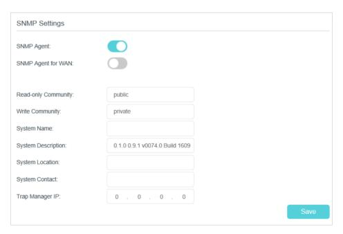
SNMP Agent: Toggle On to enable the built-in SNMP agent that allows the router to operate as the operational role in receiving and processing of SNMP messages, sending responses to the SNMP manager, and triggering SNMP traps when an event occurs.
