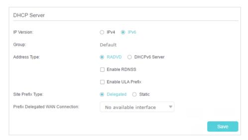
1) Select the RADVD address type to make the modem router assign IPv6 address prefixes to hosts.
