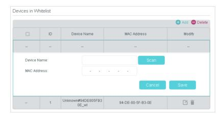
3) Click Scan and select the device from the connected device list. The Device Name and MAC Address will be automatically filled in. Or you can enter the Device Name and MAC Address manually.
