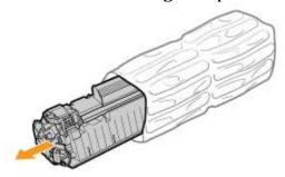
4. Shake the toner cartridge five or six times as shown in the figure to evenly distribute the toner inside the toner cartridge.
