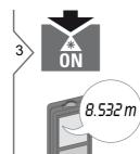
Target surfaces: Measuring errors can occur when measuring to colourless liquids, glass, styrofoam or semi-permeable surfaces or when aiming at high gloss surfaces. Against dark surfaces the measuring time increases.
