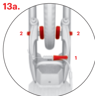
Adjusting the rear brake (V-brake)
