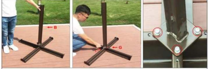
Step2. Place the tube (B) onto the cross base with bolt (G), tighten the bolt with part (1).
