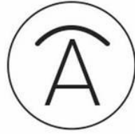
Over current protection
