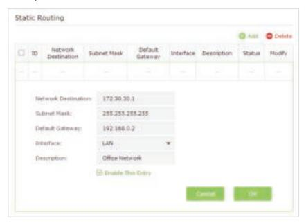
Network Destination: The destination IP address that you want to assign to a static route. This IP address cannot be on the same subnet with the WAN IP or LAN IP of the router. In the example, the IP address of the company network is the destination IP address, so here enter 172.30.30.1.
