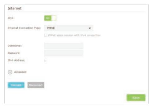
4) 6to4 Tunnel: An IPv4 Internet connection type is a prerequisite for this connection type (*Manually Set up Your Internet Connection*). Click Advanced to do more configuration if your ISP requires. Click Save and then click Connect to finish the configuration.
