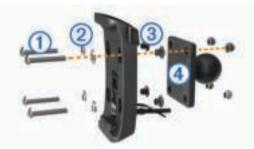
2 Tighten the nuts to secure the base plate.
