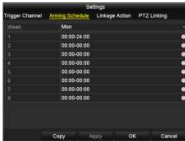
Figure 8-6 Set Arming Schedule of Alarm Input
