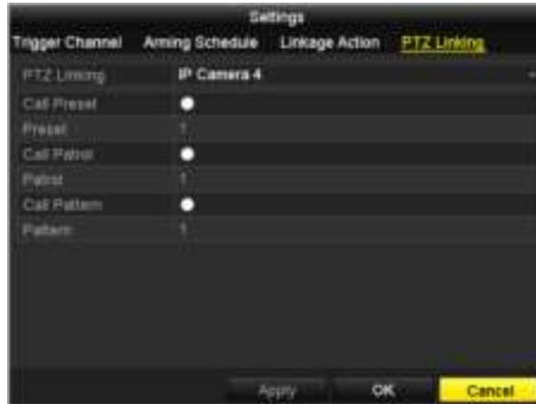
Figure 8-7 Set PTZ Linking of Alarm Input
