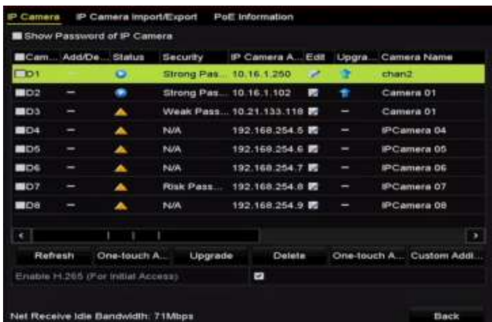
Figure 2-25 IP Camera Management Interface
