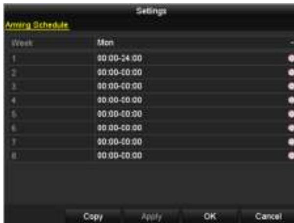
Figure 8-17 Set Arming Schedule of Alarm Output
