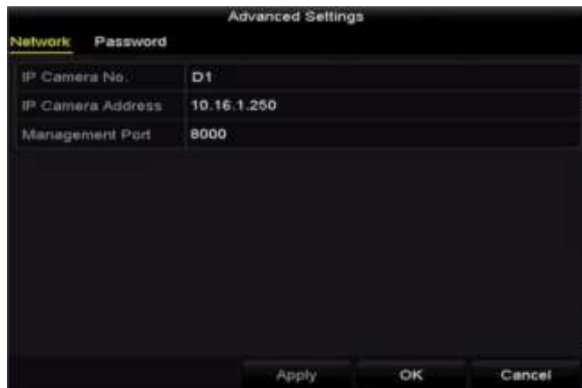
Figure 2-36 Network Configuration of the Camera
