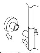
Step 6 Remove the riser and the mounting piece.
