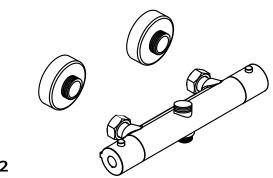
Step 2 Install the main body and rubber pad.
