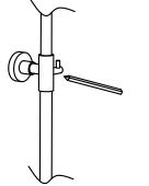
Step 5 Makesure the riser is level, mark the position of the screw holes.
