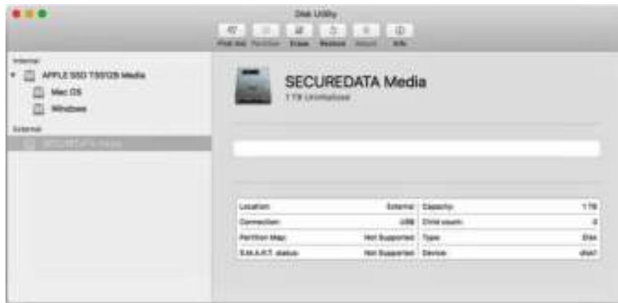
Figure 3: The Disk Utility Dialog. Make sure the correct drive is highlighted (There is only one External drive listed in this image).
