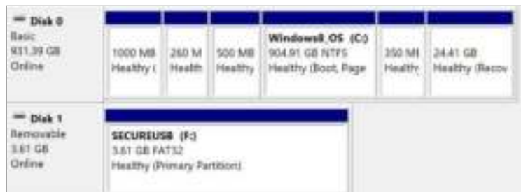
Figure 2: The SecureUSB is displayed here as "Disk 1." It is Online and allocated (Healthy) and ready for use.
