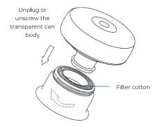
After replacing the attached filter cotton, Restore and install the transparent can body.
