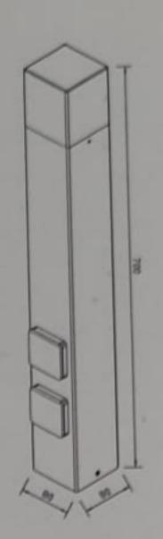
OUTDOOR LIGHT WITH DAYLIGHT SENSOR ALW7937-700-2SC IP44 220-240V 50Hz
