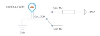
• When the output is on, the COM and N/O terminals will be internally connected to each other. Here is a schematic of the output circuit:
