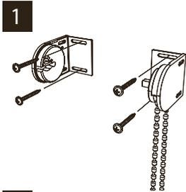
The first step is to mark the holes where you are going to put your screws. Determine how far apart your holes should be.
