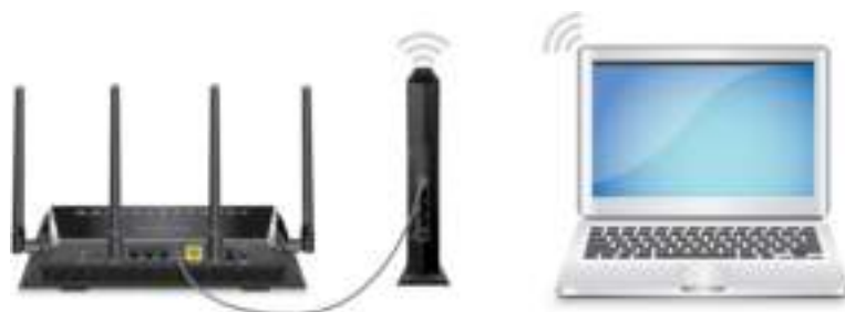
Figure 4. Extender in access point mode
