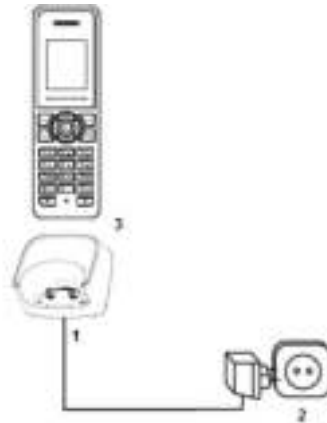
Figure 6: Setting up the charger station
